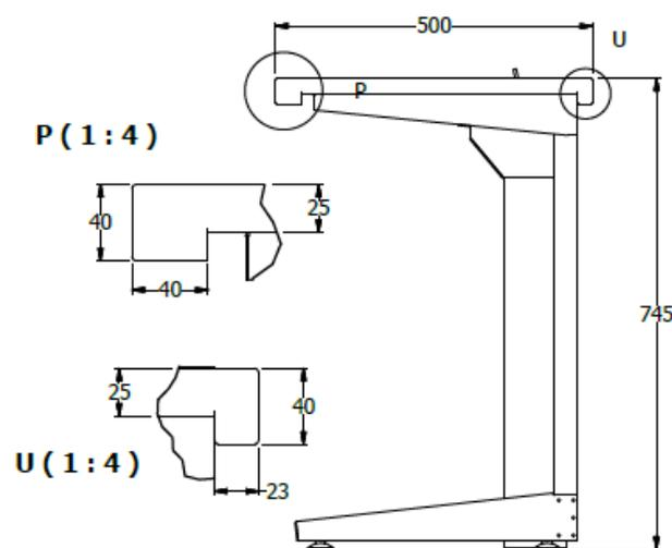
MESON DE TRABAJO ENTRE COLUMNAS ESP. 0,73X5,44X0,50 MELAMINA 25MM CONTORNO 50MM
